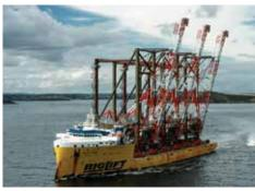
Three Liebherr ship to shore container cranes on their way to the USA after partial assembly in Ireland
